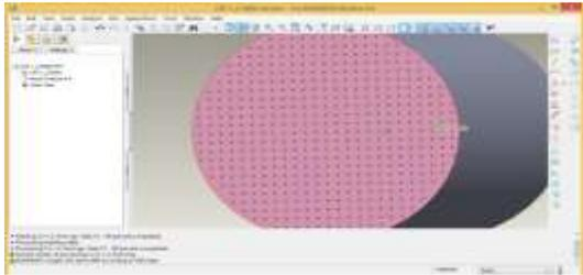
**Design of circular cells of 1.2mm size and 5mm distance between channels**
