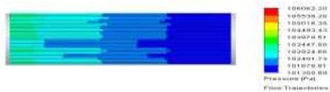
Pressure drop for 1.5mm and 4mm distance between circular channel at 20m/sec
