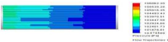
Pressure drop at 1.5mm and 4mm distance between square channel at 10m/sec
