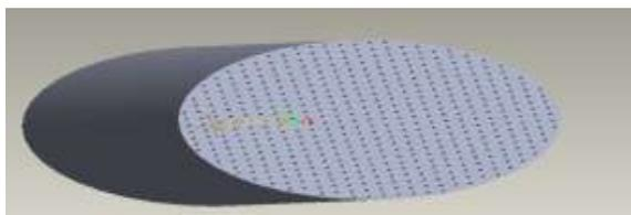
**Design of circular cells of 1.5mm size and 5mm distance between channels**
