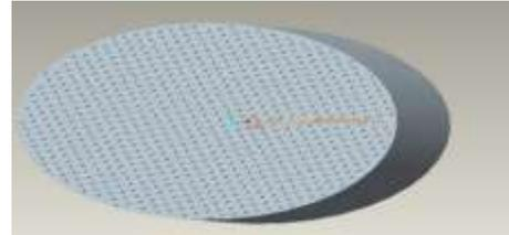
**Design of Triangular cells of 1.5mm size and 4mm distance between channels**
