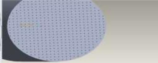
**Design of circular cells of 1.2mm size and 4mm distance between channels**
