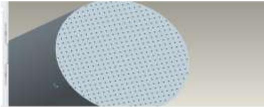
**Design of square cells of 1.2mm size and 4mm distance between channels**
