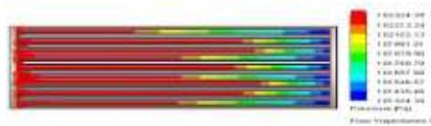
Pressure drop for 1.5mm and 5mm distance between Triangular channel at 20m/sec
