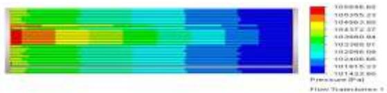
Pressure drop for triangular channel of 1.2mm size and 5 mm distance between channels at 20m/sec
