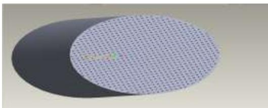
**Design of circular cells of 1.5mm size and 4mm distance between channels**
