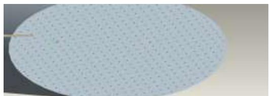
**Design of triangular cells 1.2mm size and 4mm distance between channels**
