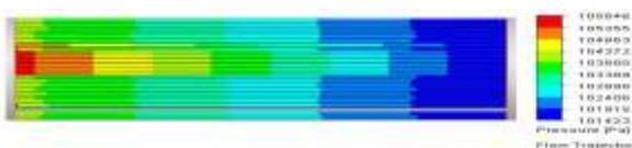
1.2mm size and 5mm distance between square channel Pressure Drop at 10m/sec
